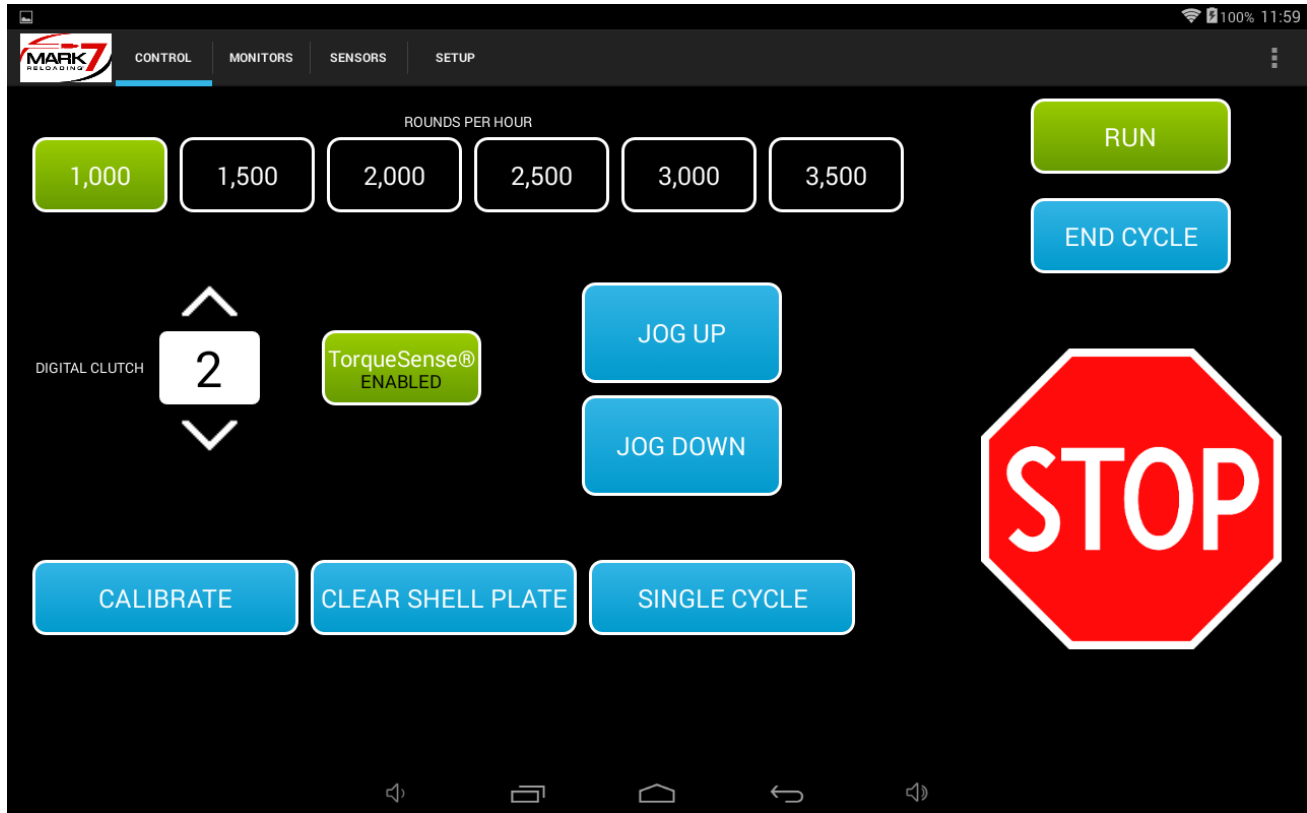
Figure 22: System Control Screen.
