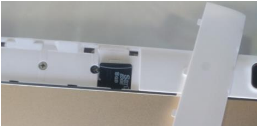
1. Proper Insertion of micro SD card into Gold tablet.
