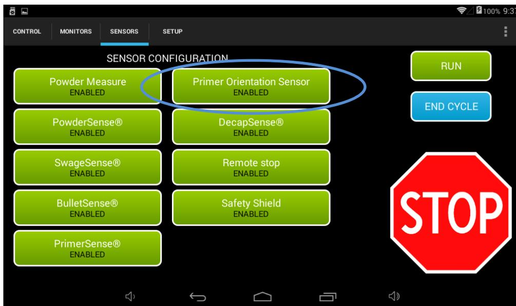
Figure 1 : Enabling Sensor
