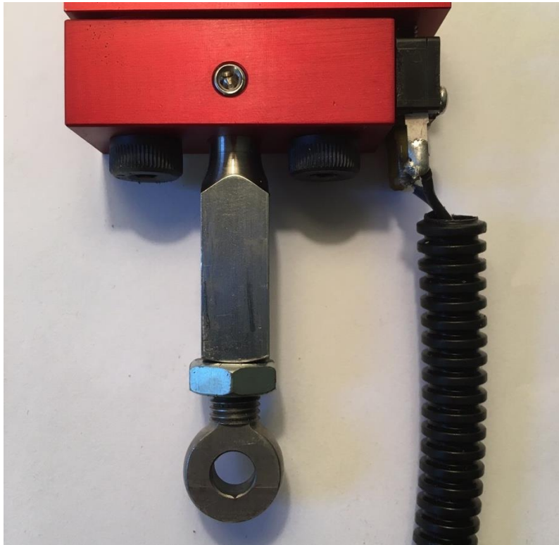
Figure 30: Rod end installed
