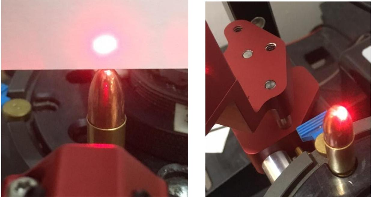
**Figure 43: Beam Over Bullet (Left) the Reflected Beam Will Hit the Back of the Bullet (Right)**
