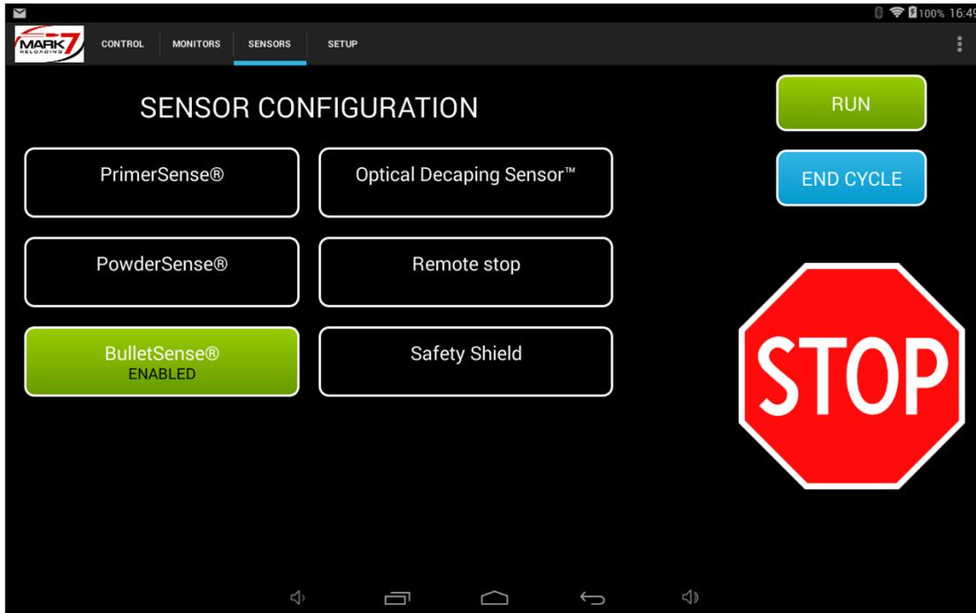
Figure 45: Enabling BulletSense® on Sensor tab
