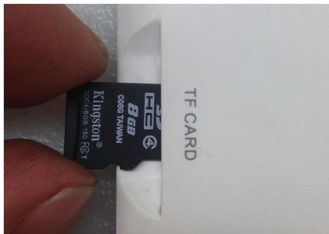
Figure 53: Orientation of Micro SD card
