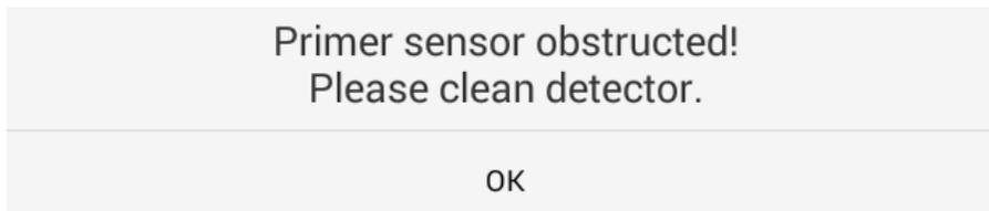
In either case the recommended cleaning interval is every 500-700 rounds that are decapped. Using a duster can or compressed air, spray into spent primer hole in the 650 platform and into the front hole on the decap sensor shown below. It may be necessary to remove the sensor.
