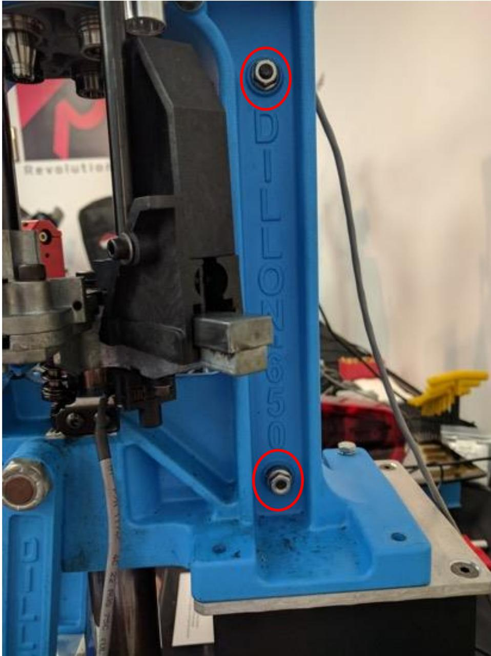
Figure 37: Case Feeder Mounting Bolt Locations
