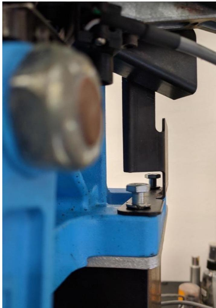
**Figure 36: Removing offload bracket**
