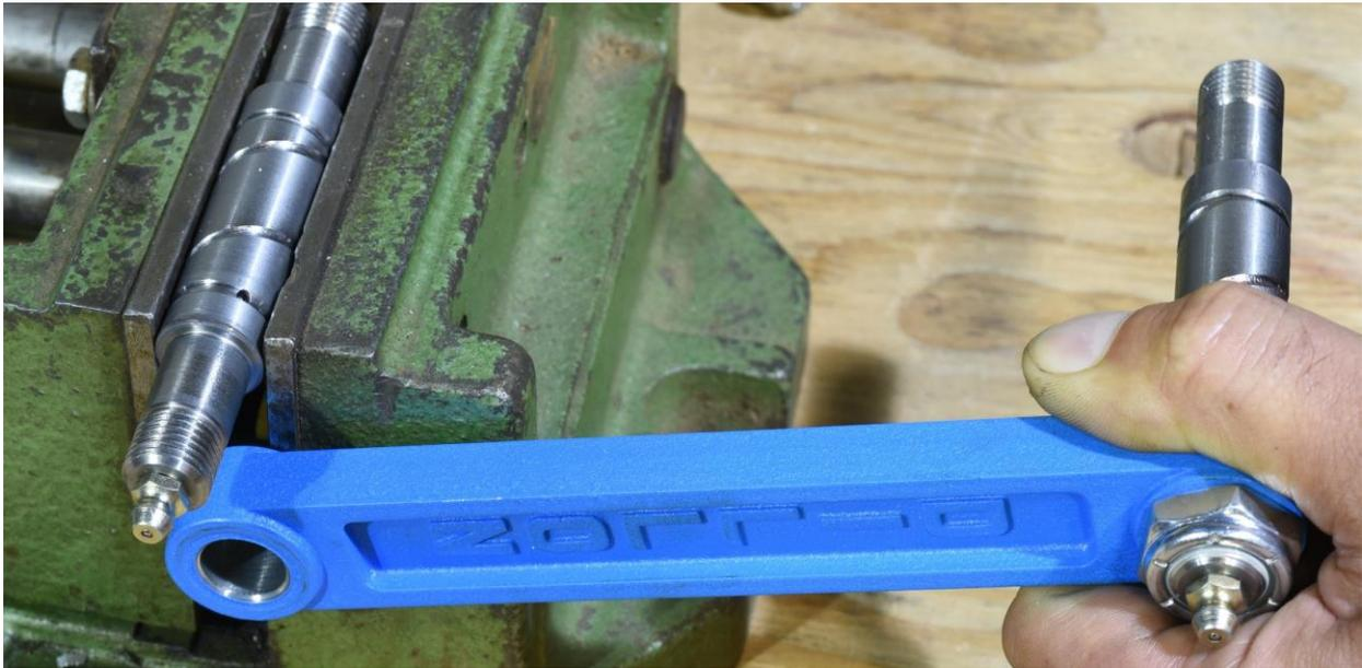
Figure 10: Left Link Removed
