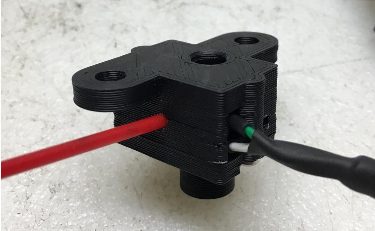
Figure 32: Blowing Out Decapping Sensor with Compressed Air.
