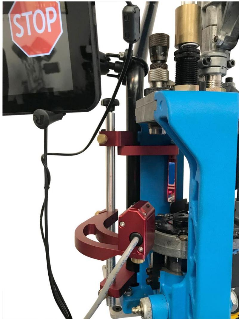
**Figure 40: Lining Up Laser with Mirror (Crude Adjustment)**
