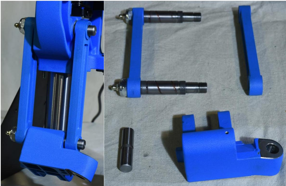
**Figure 8: Link Arms, Knuckle and Pin Removed From 650.**
