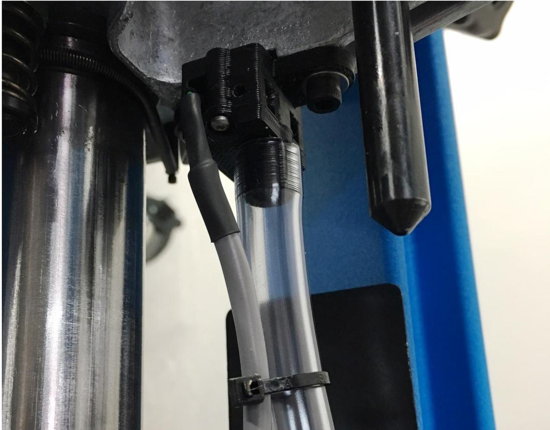
**Figure 31: Decapping Sensor Installed**
