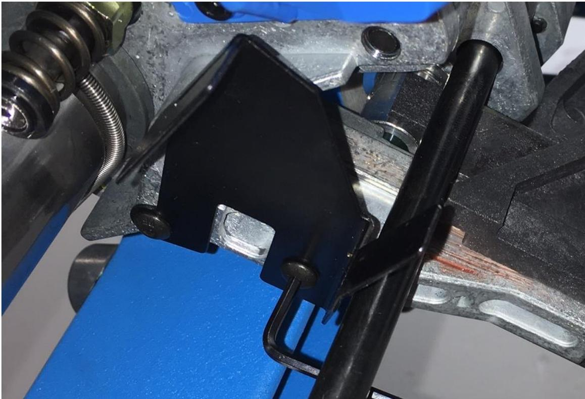
Figure 30: Removing 650 Primer Bracket
