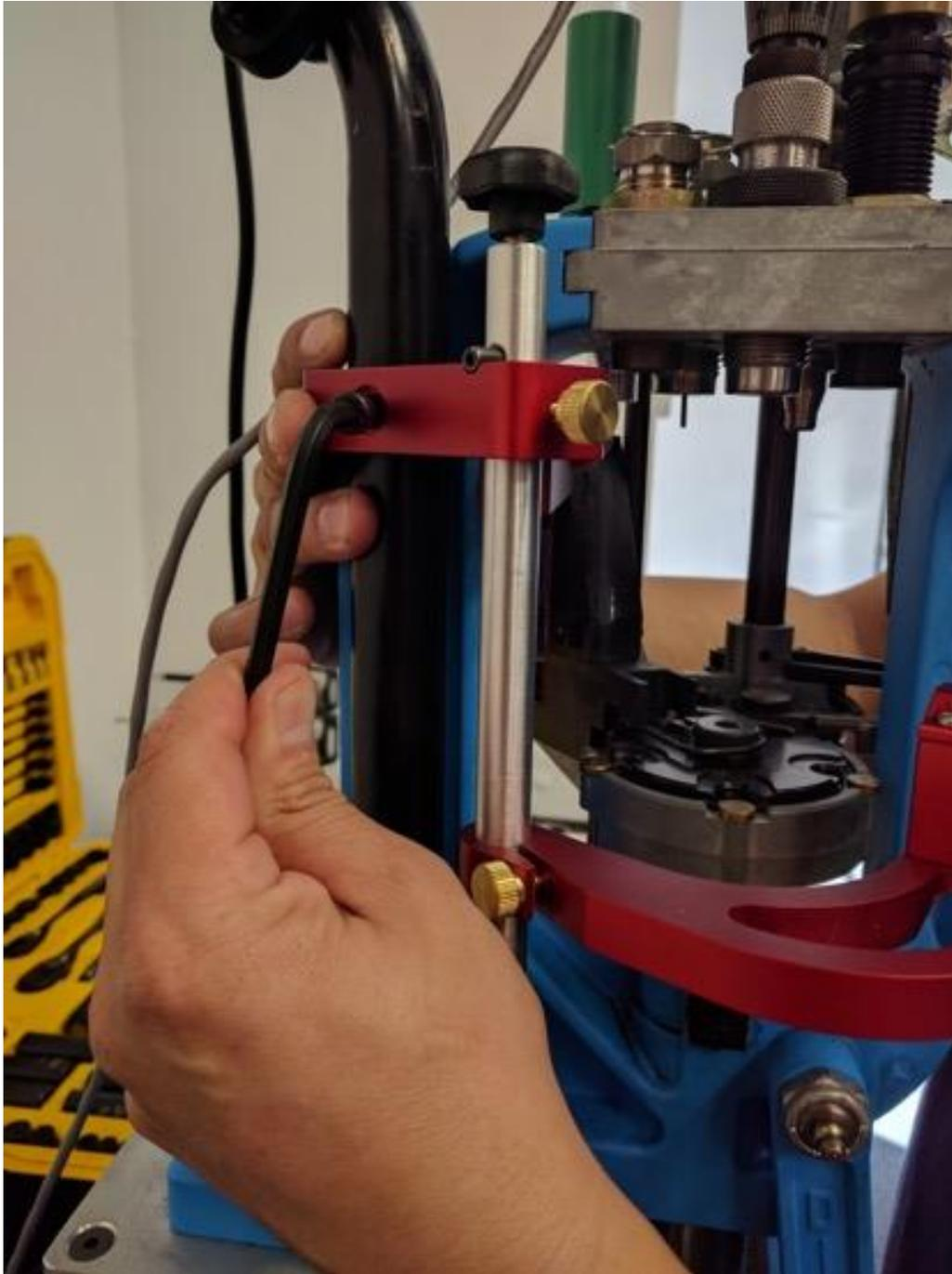
**Figure 38: Installing BulletSense® on XL 650.**
