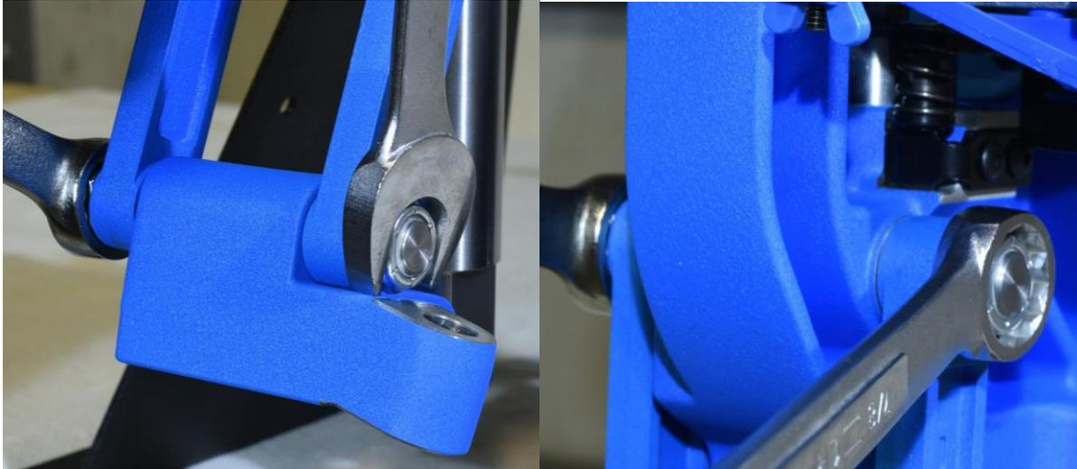
**Figure 7: Removing Link Arms (Remove Left Link Arm)**
