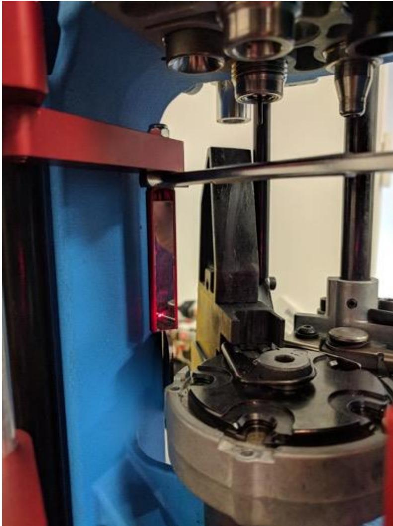
Figure 39: Installing Mirror Bracket
