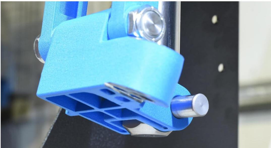
Figure 6: Removing Knuckle Pin (Do not Discard Pin)
