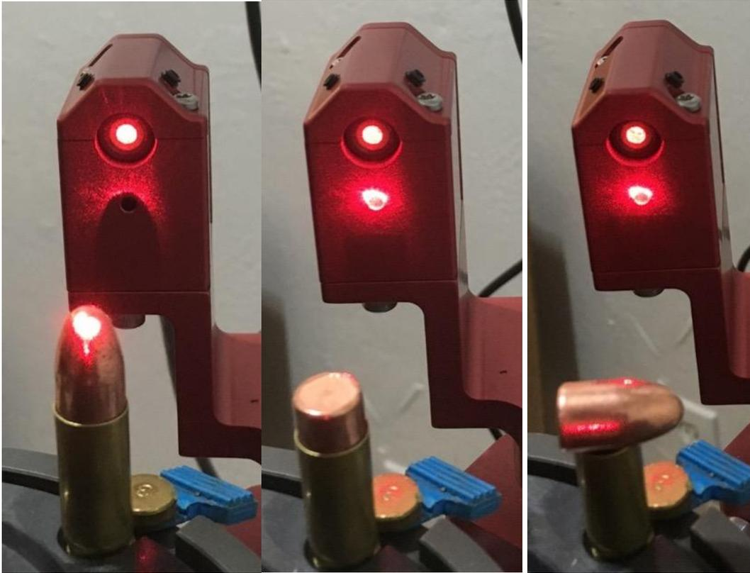
**Figure 44: Bullet Properly Oriented - Beam Interrupted (Left)**
