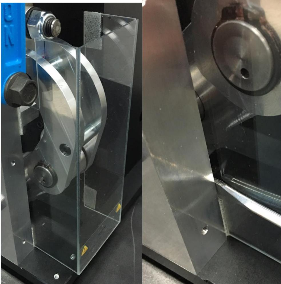
**Figure 18: Shield Installed (Left). Removing Shield (Right)**
